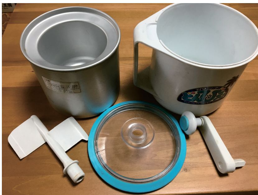
Photo 1 Components of a Donvier frozen vessel home-use ice cream maker model for making about 500 ml of ice cream. Front L to R: dasher, lid, crank handle. Back L to R: aluminum vessel containing refrigerant within its double walls, outer vessel. Duell photo.
