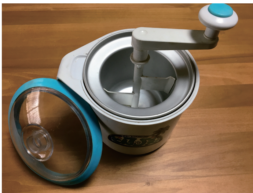
Photo 2 Assembled components of Donvier frozen vessel home-use ice cream maker. After pouring in ice cream mixture and closing lid, dasher is hand-cranked occasionally for about 15 minutes to yield about 500 ml of ice cream. Duell photo.
