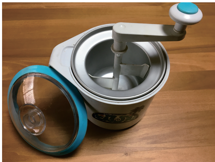
Photo 2 Assembled components of Donvier frozen vessel home-use ice cream maker. After pouring in ice cream mixture and closing lid, dasher is hand-cranked occasionally for about 15 minutes to yield about 500 ml of ice cream. Duell photo.
